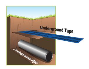
A typical excavator starts with a shallow cut to mark the spot and check for obstructions. for maximum early benefit this tape should be buried no deeper than 6-10" below grade. The wider the tape the greater the detection capabilities and visibility.
