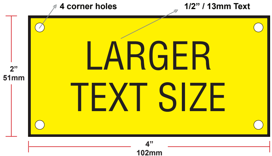
Illustration 2: Nameplate for viewing distances of 72" (1830 mm)
