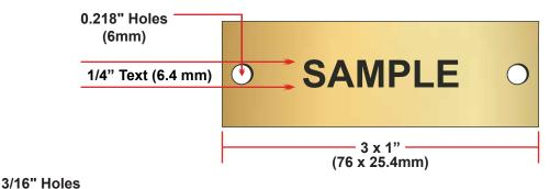
Illustration of nameplate for viewing distances of 72" (1830 mm)
